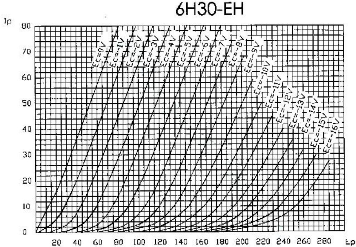
The 6H30 is a medium mu dual triode with a very high-pervenance cathode. The low plate resistance, combined with superior linearity, and a true 4 watt per plate dissipation, make for a high performance voltage amp or driver.
