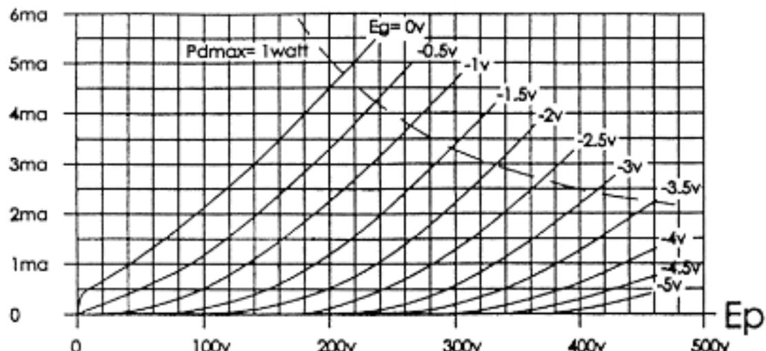
The 12AX7EH is a dual high mu triode with a spiral filament and special construction to minimize microphonic behavior. Ideal for replacement use in guitar amps and any place low noise and high gain is important.
