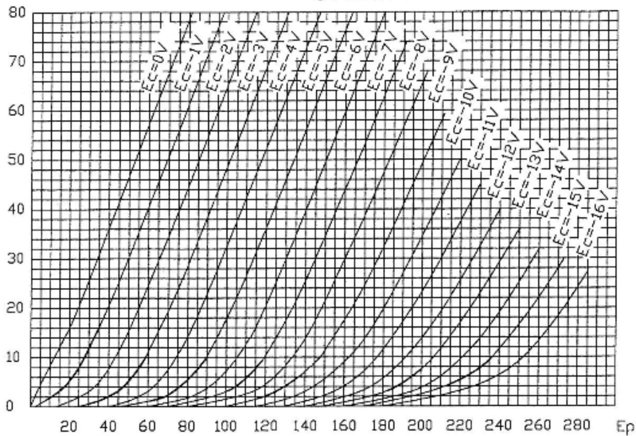
The 6H30 is a medium-mu dual triode with a very high-pervenance cathode. The low plate resistance, combined with superior linearity, and a true 4 watt per plate dissipation, make for a high performance voltage amp or driver.
