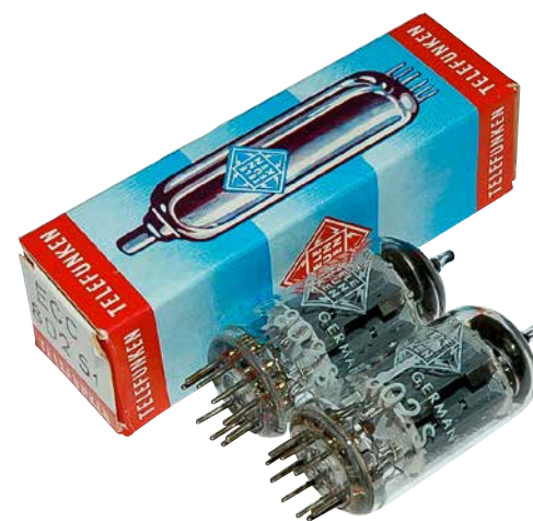
▲ Two desirable pearls in the form of the double triode ECC802S, an especially durable Telefunken tube. It has been off the market for a long time but BTB keeps buying residual stock – at three-figure prices.
